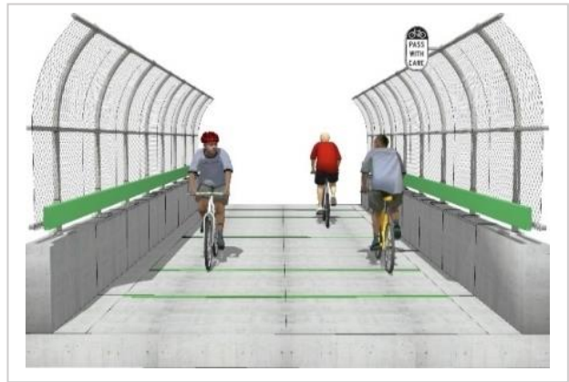
ADA-compliant 14' wide sidewalk access ramp, maximum 5% slope (11' wide at NJ north)
